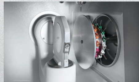
Cleaning-friendly design of the milling chamber and resistant water-repellent coating
